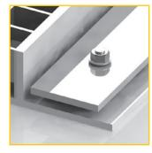
Loose/fixed flange all around, material thickness 6 mm. Solid threaded bolts M12 with spacing of 150 mm ensure a reliable compression of the gasket sheet with the help of the 60 mm wide loose flange.
